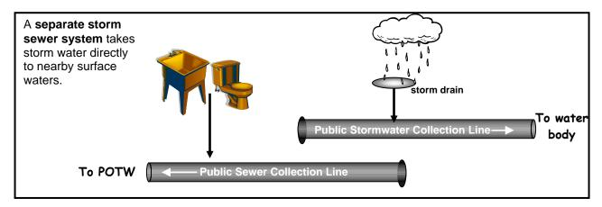
Figure 2: Separated Sewer System
