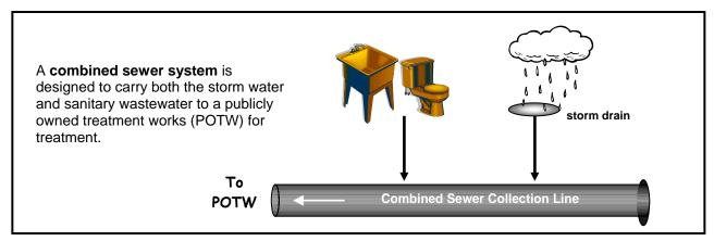
Figure 1: Combined Sewer System
